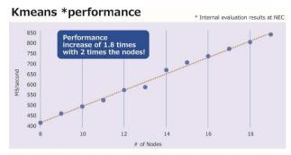
\* Kmeans: One of the Hibench benchmark tests for determining the Hadoop/Spark performance index. With this performance index for processes used in areas such as machine learning, randomly allocated data is classified based on the measure of similarity between data.
