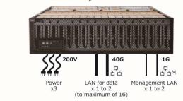
Add servers simply by inserting server modules into the chassis. Since the platform supports hot-swap, you can add servers and replace defective servers without shutting down the entire system. There are 3 power sources built in to the chassis, and fan modules are configured redundantly, so there is no need to stop operation while recovering from failures.
